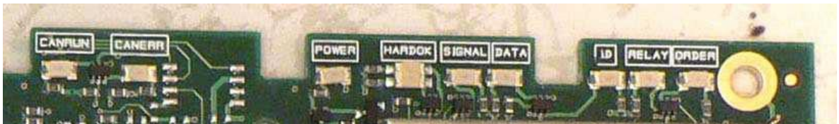
Figure 5. Signalling LEDs in the receiver.
